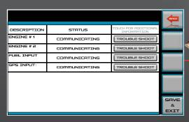
**Engine Monitoring** – for J1939 or NMEA2000 protocol for up to 5 engines.
